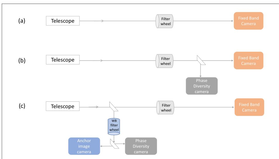
*Figure 1. Conceptual design for the EST FBIs. (a) The simplest setup: one camera and a filter wheel with narrowband filters. (b) As (a) plus a beamsplitter and a synchronised, defocused camera for Phase Diversity. (c) The chosen setup, as (a) plus a Phase Diversity pair of cameras behind a wideband filter wheel. Graphics courtesy C. Quintero Noda.*
