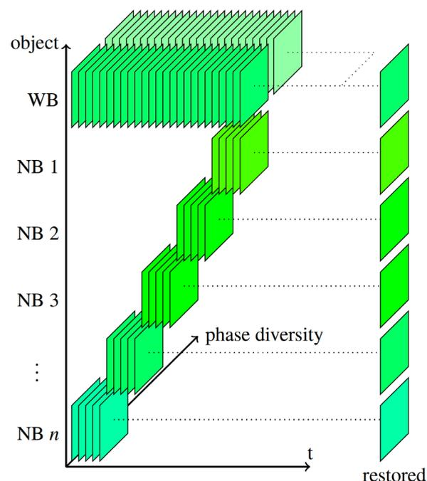
Figure 3. Schematic representation of a MOMFBD dataset with Phase Diversity. The WB images force MOMFBD to align the restored NB images.
