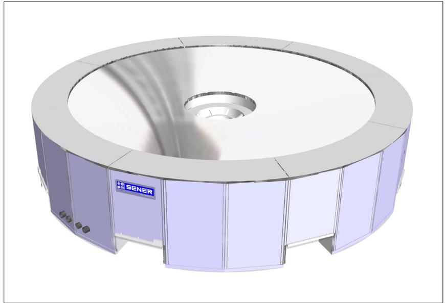
*3D model of the EST primary mirror and supporting mirror cell. Credit: SENER*
