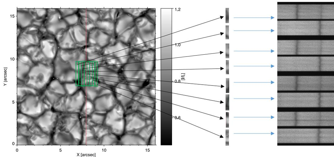
Figure 2. illustration of how an IFS based on image slicers works. Multiple sub-slits (green on the left) record a small FOV (middle), and a given spectral range over that FOV (right). Image credit: Silvia Regalado Olivares (IAC).
