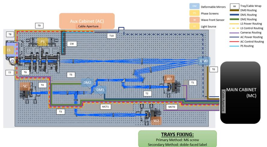
Figure 1. EST MCAO testbench (top) and schematic (bottom). Credit: C. Quintero/IAC
