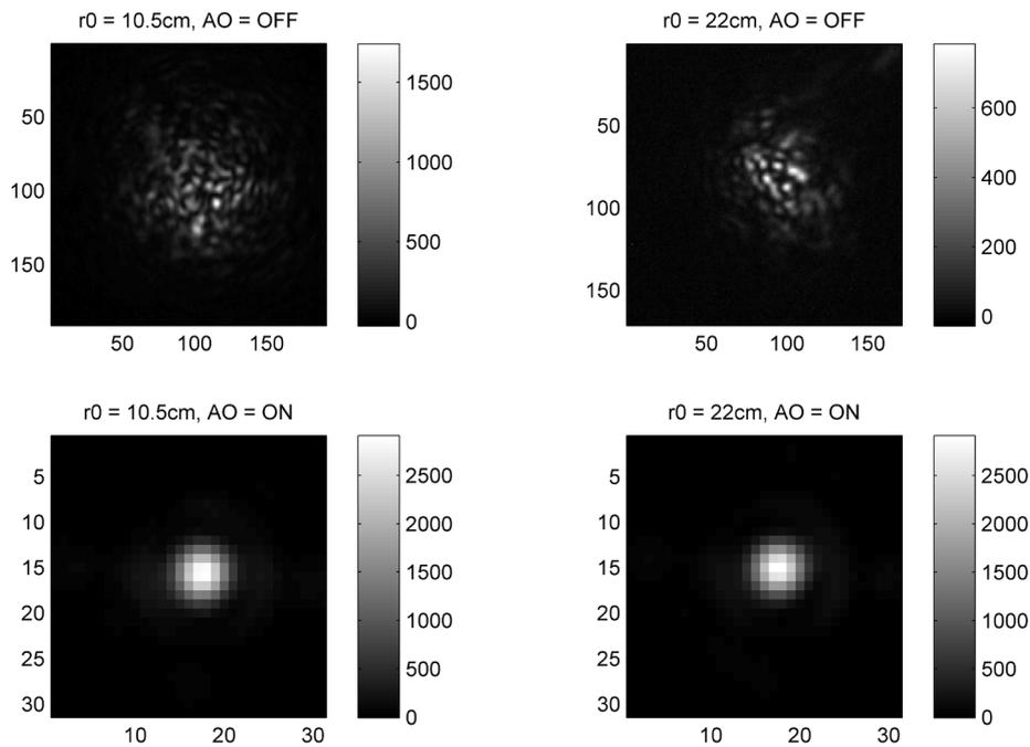
Figure 2. Point spread function (PSF) of the uncorrected wavefront for  $r_0 = 10.5$  cm (left) and  $r_0 = 22$  cm (right), and best corrected PSF achieved (top and bottom panels, respectively)
