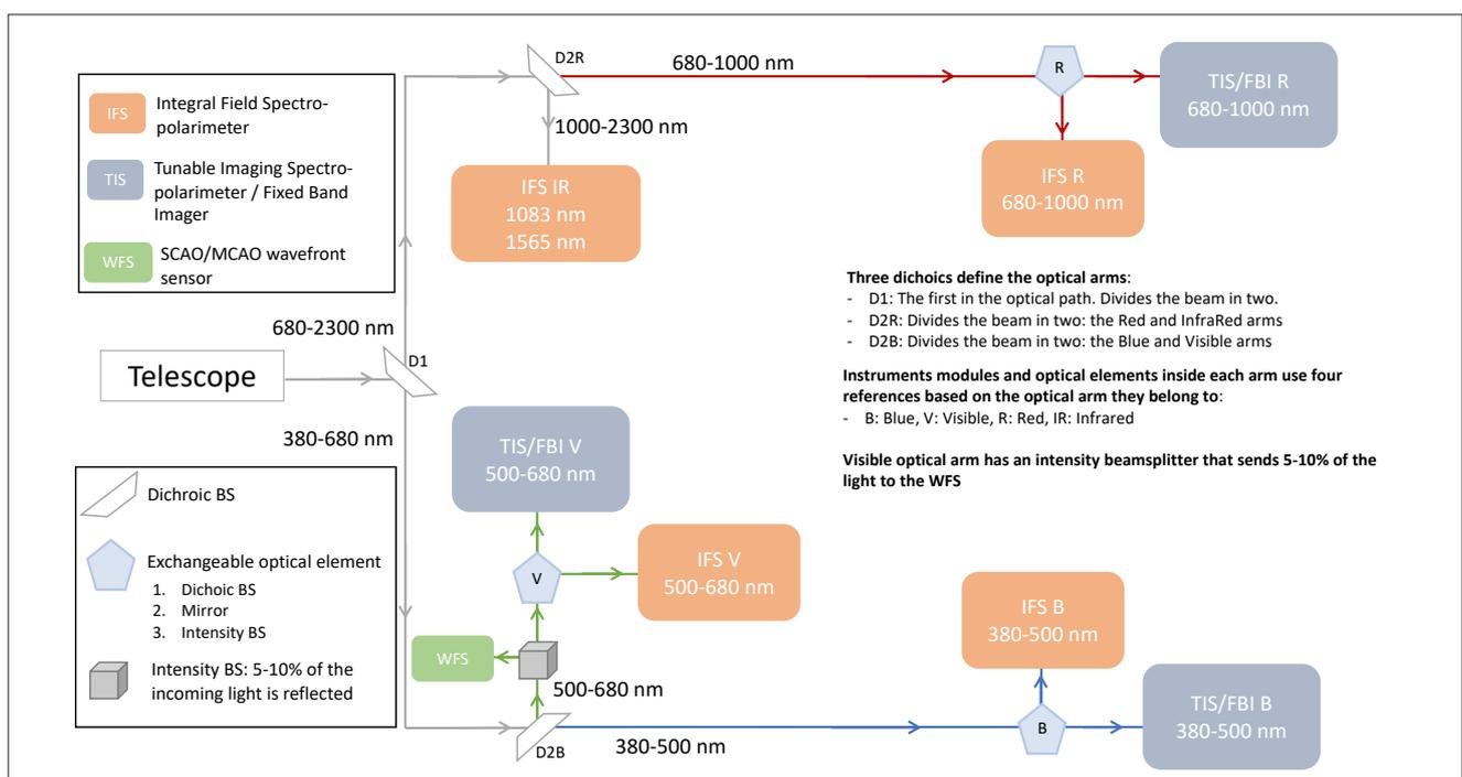
Current concept of the EST instrument suite, based on Tunable Imaging Spectropolarimeters and Integral Field Spectropolarimeters
