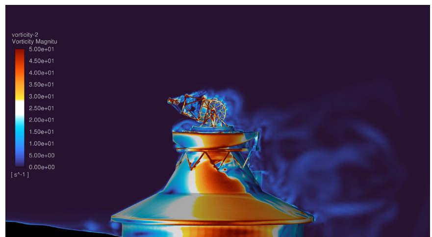
Fig. 2. Vorticity in a vertical plane containing the telescope optical axis.
